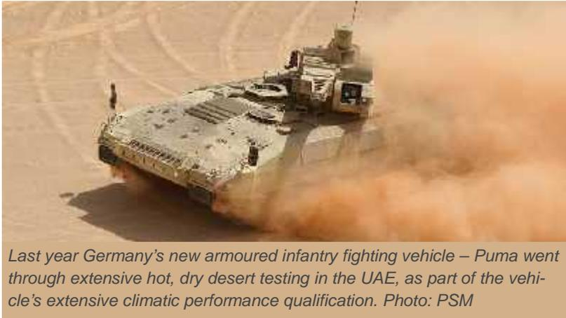
*Last year Germany's new armoured infantry fighting vehicle – Puma went through extensive hot, dry desert testing in the UAE, as part of the vehicle's extensive climatic performance qualification. Photo: PSM*
