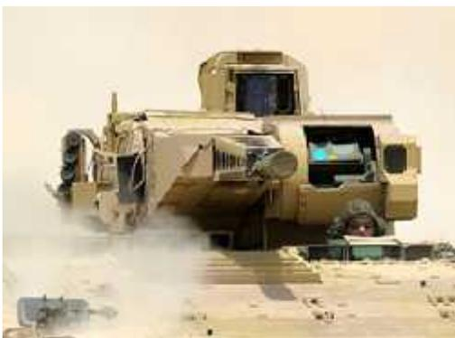
*Among the vehicle's unique attributes are its effective modular protection concept, a remote-control, stabilized turret armed with an ABM capable 30mm automatic cannon, and decoupled running gear with hydro-pneumatic shock absorber elements. Photo: PSM*
