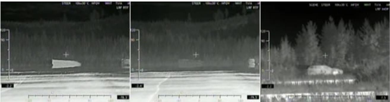
ADAPTIV can instantly blend a combat vehicle into the background, reducing detection range below 500 meters.
